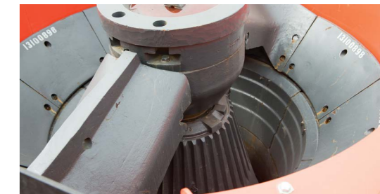
MC chamber with extremely large feed opening
