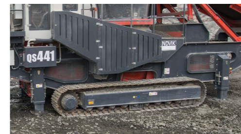
Four jacking legs for increased servicing capabilities
