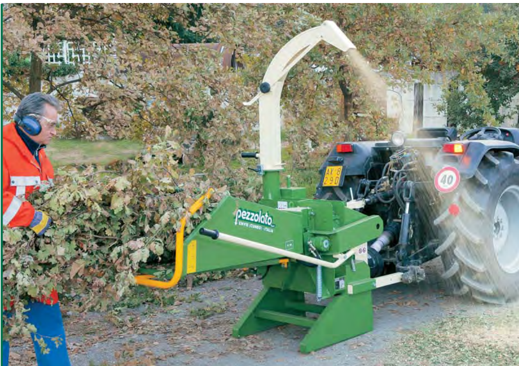
The PZ 100 G version at work, driven by PTO and equipped with attachment to the 3-point hitch of the tractor.
