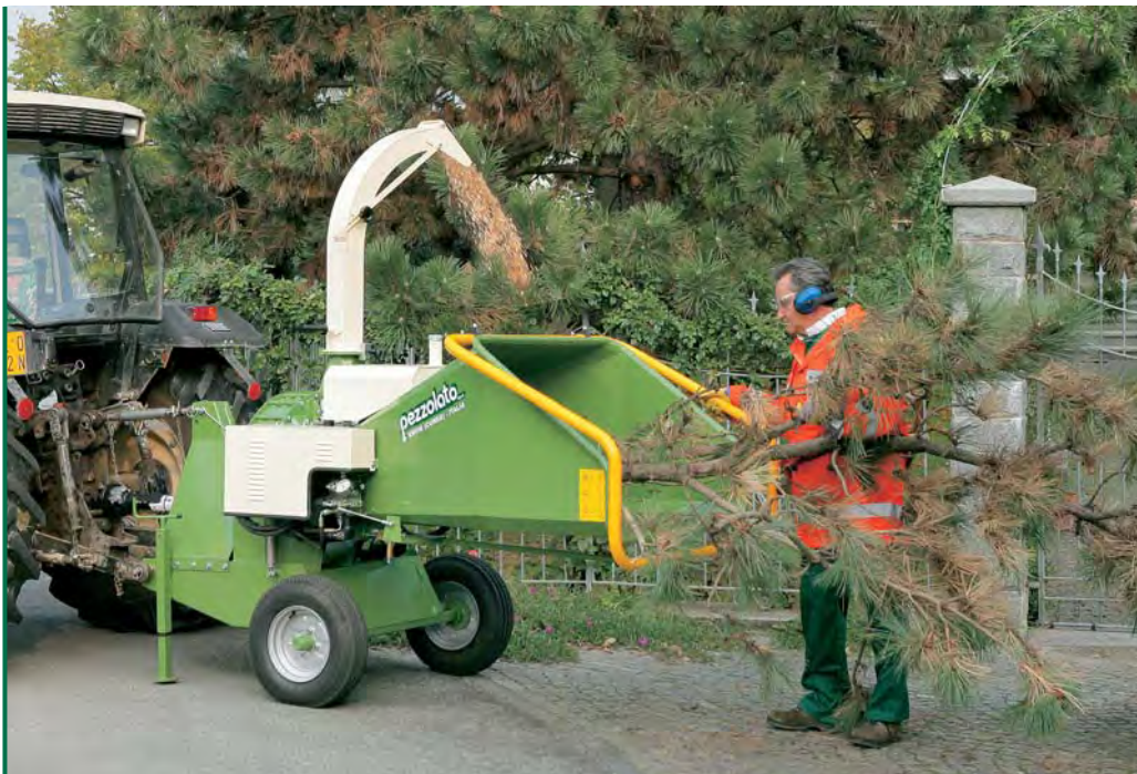
The PZ 140 G version at work, is driven by PTO; it has a 3-point hitch and rubberised wheels to ease storage. By applying the removable bar the machine can also be towed at low speed.
