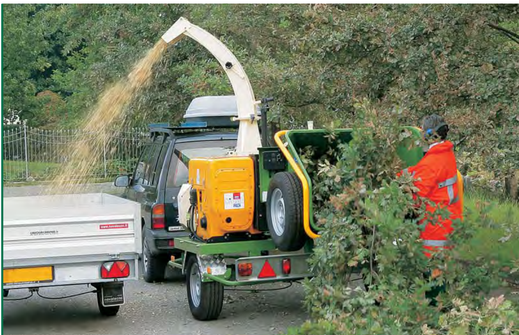
The PZ 190 M version at work. It is driven by a silenced HATZ 52 Hp Diesel engine, mounted on a trailer for 80 km/h. Also this machine – on request – can be mounted on a “tandem” trailer with rotating platform.
