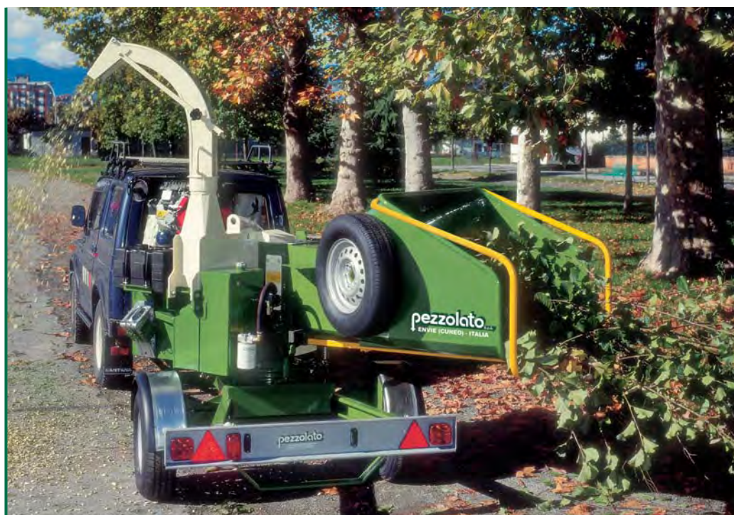
The PZ 150 MB version at work. It is driven by a 20 Hp petrol engine and mounted on a trailer for 80 km/h. It has a rotating platform that allows to position the feeding hopper in a way to ease entry of the material to be chipped to a maximum.
