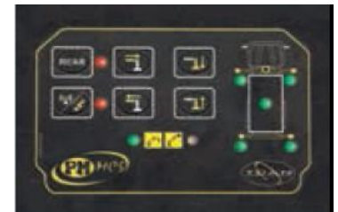
Remote controlled outriggers and MCS system
