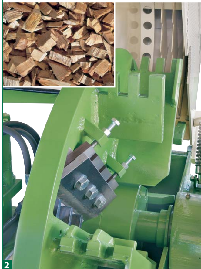
1 Detail of the material feeding mouth; the feeding rollers are visible on the base and, in the background, the disc with a chipping knife. Roller speed can be adjusted by the operator, in relation to the type of material to be chipped.
