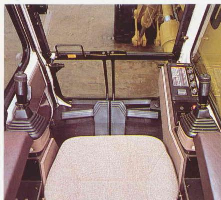
**Human engineered cab:** The large tinted glass windows provide excellent all-round visibility. Windows open wide to provide plenty of ventilation. The 5-way fully-adjustable reclining seat has armrests and suspension-mounting for additional comfort.
