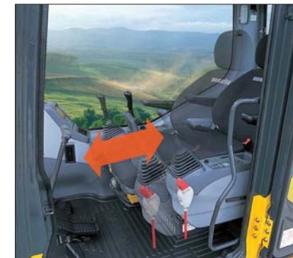
Seat Sliding Amount: 340 mm 13.4", increased 120 mm 4.7"
