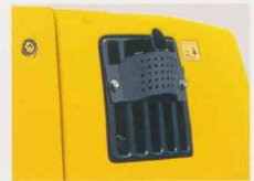
Upward exhaust pipe
