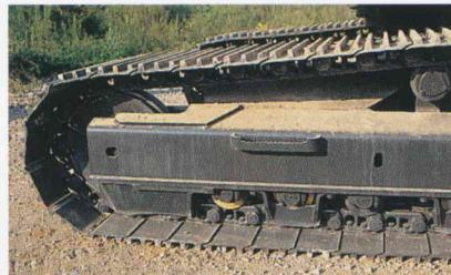
The track link pitch has been enlarged to the next size class, and a strut has been added for increased durability.
