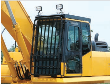
Cab with two-piece pull-up window
