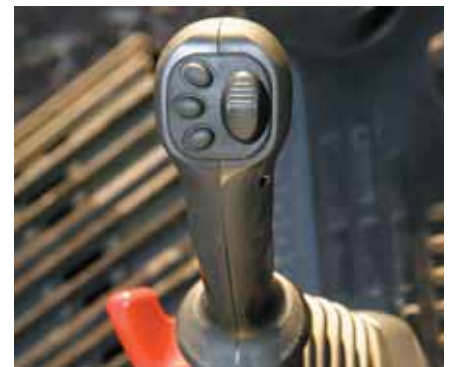
Joysticks with proportional control button for attachments
