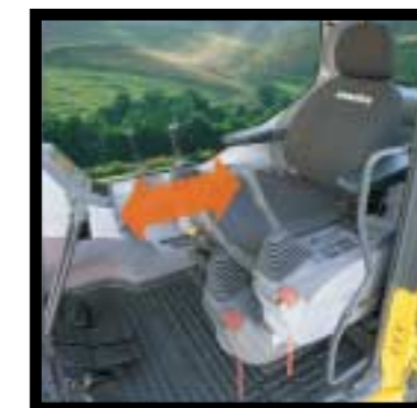
Seat Sliding Amount: 340 mm 13.4", increased 120 mm 4.7"
