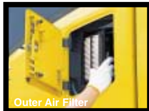
Removal and installation of air conditioner filter element, without tools, facilitates cleaning.
