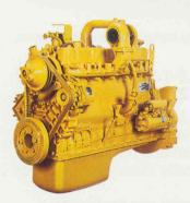
Komatsu S6D105 — provides 148 HP and 6.49 ltr. (396 in³) displacement. The S6D105 is a 6-cylinder, direct injected, water-cooled, turbodiesel that operates both quietly and efficiently.
