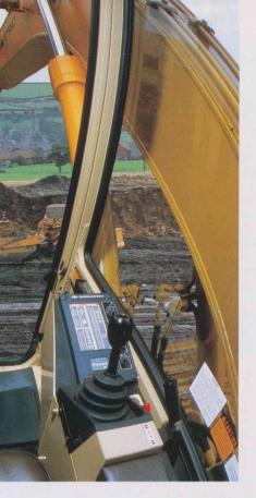
Travel/steering controls: are foot pedals with detachable lever controls. Either can be used depending on application and operator preference.
