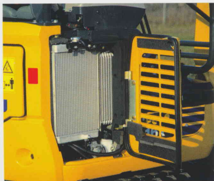
Right bonnet: simple inspection and cleaning of the radiators
