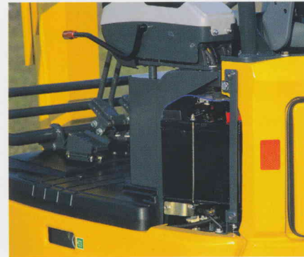
Left bonnet: easy access to the battery
