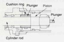
**Cushion mechanism** — in the arm cylinder and head end of boom and bucket cylinders absorbs operating shocks from cylinder extension and retraction, increasing both operating comfort and component life.
