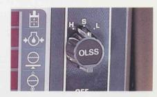
digging and loading and the Light-Duty mode enables the operator to maintain quick cycle times and save fuel during light operations (such as slope finishing).
