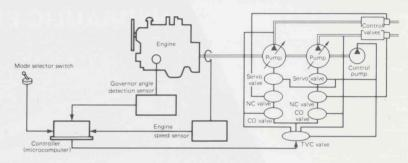
**Electronic Open-center Load Sensing System (EOLSS)** — electronically controls oil flow from the three variable capacity piston pumps so that unnecessary oil flow can be eliminated and fuel consumption significantly reduced. A microcomputer matches oil discharge volume to engine speed (even at high altitudes) so that engine ouput power can be effectively utilized. This also reduces fuel consumption since the engine is not generating unused power.
