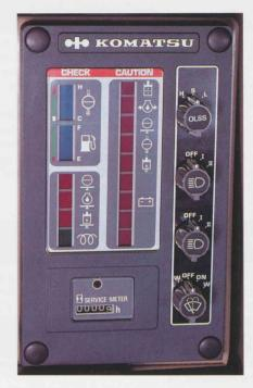
**Electronic monitoring system** — is a display panel that continuously monitors all operating systems. If a malfunction should occur, the operator is immediately warned which system is experiencing trouble, saving valuable time lost searching for the problem. Also, gauges constantly monitor service hours, engine water temperature and fuel level.
