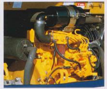
Komatsu-built 3D75 engine provides a tenacious power of 17.8 HP (14 kW) at 2600 RPM. Its large piston displacement assures powerful excavation even at partial throttle, without fear of stalling.
