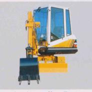
**Convenient boom offset:** The boom itself can be swung 57.5° to left and right. This means that the PC10-5 can complete quick dig/load operations in extra tight quarters without swinging the upper structure of which the tail end may hit obstacles such as walls, poles, etc.(Steel cab is optionally available.)
