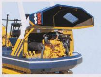
**Full-open machine cover** allows quick access to internal components such as engine, hydraulic equipment, etc., for both quick checking and repairing.
