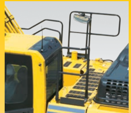
Hand rails and anti-slip plates
