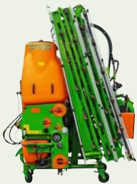
UF mounted sprayer, 900, 1,200, 1,500 and 1,800 litres, 12 to 28 m
