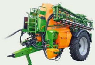
UX trailed sprayer, 3,200 - 4,200 - 5,200 - 11,200 litres, 15 to 40 m
