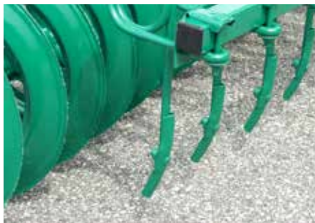
16mm front finger harrow with reversible point.
