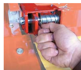
Quick-change pins for conditioner
