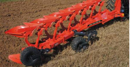
The wheel is equipped with a central pivot allowing it to automatically follow any changes in working width. The depth is adjusted by turnscrew (1) (or hydraulically 2) with the possibility to adjust the depth differently on each side. The depth wheel can be mounted in many different positions along the beam in order to achieve the best possible configuration.
