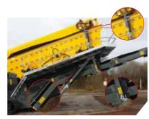
**Easy Change of Screen Media**Drop tail conveyor and screen-box to the ground for ease of access.
