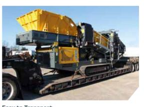
Scalper can be moved in one piece without disassembling catwalks.
