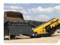
**Large 12yd<sup>3</sup> Feed Hopper**Designed to be fed with wide loader buckets.
