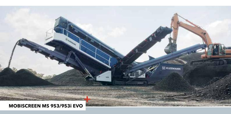
The mobile screening plant MOBISCREEN MS 953 EVO is equipped with a 9.5 m<sup>2</sup> screen box. The triple-deck screening plant impresses with a feed capacity of up to 500 t/h. It is operated by a modern control system. All functions are thus easy to control, operating statuses and machine functions can be viewed at any time.
