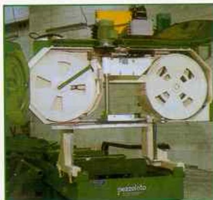
**Professional horizontal band sawmill**, heavy duty quality for multi shift work, for all kind of wood up to 1,2 m log diameter, fully hydr. operated, cutting length from 6,1 m, productivity approx. 3,5 - 4,5 m<sup>3</sup>/h, alternatively electric- or diesel drive. Standard equipment: 5 log grips, 2 driven taper adjusters, 1 log turner, 2 squaring arms. Optional equipment: computer operating, debarker unit, board remover arm, log loading arms, precutting saws, cross cutter.
