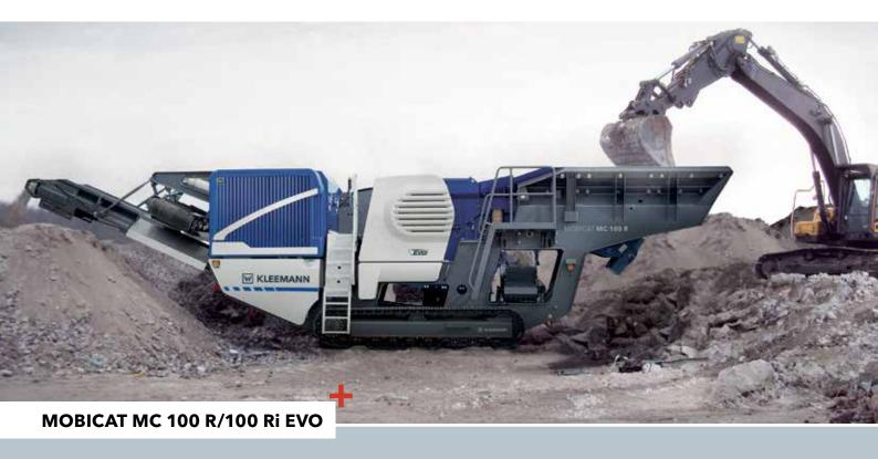
The smallest mobile jaw crusher of the EVO line impresses with its compactness and reliability. Can be used for the most varied of materials, the plant offers wide-ranging possibilities for both demolition companies and contract crushers. Thanks to diesel-direct drive, the MC 100 R EVO has a lower fuel consumption.
