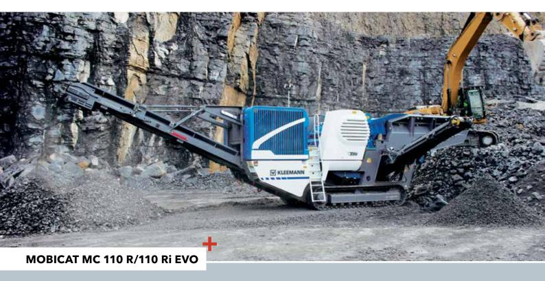
The MC 110 R EVO's advantages include considerably high power in its class and its vibrating feeder with integrated slotted grate. The plant is used as a primary crusher for natural stone as well as in demolition and recycling companies. It is lightweight, making it easy to transport and flexible to use.
