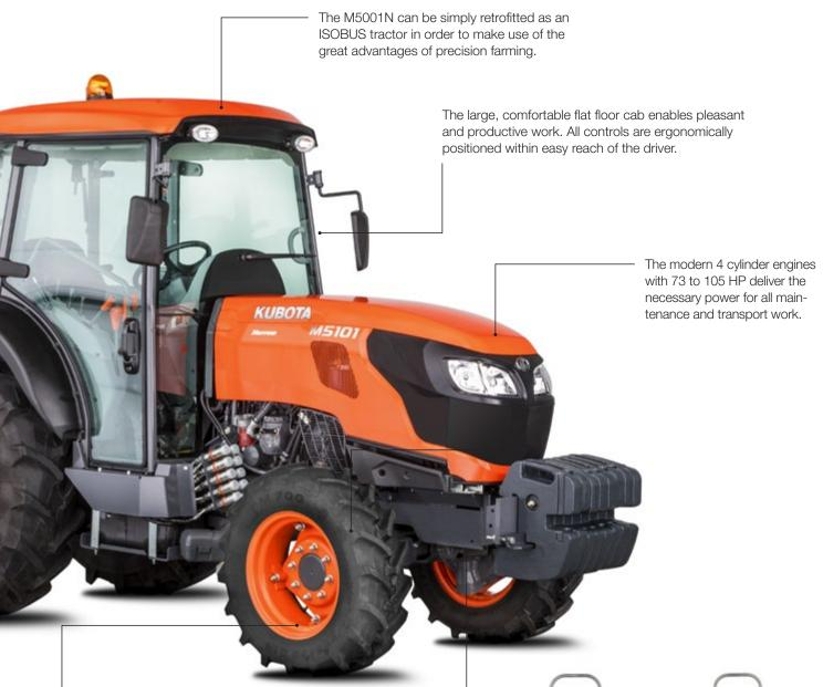
An excellent 55° steering angle and the unique "bi-speed turn" by Kubota give the tractor unparalleled manoeuvrability. This results in an excellent turning radius of 3.95 m.
