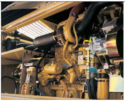
Ground Level Service. The design and layout of the M318C was made with the service technician in mind. The fuel water separator, engine oil filter, battery, radiator fluid level, fuel filter, engine oil gauge, hydraulic oil level, air cleaner and pilot system filter are all easily accessible at ground level allowing critical maintenance to be done quickly and efficiently.
