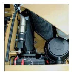
**Powerful Performance.** The 3056E DIT ATAAC engine delivers a net power of 113 kW (154 hp) at the rated speed of 2000 rpm, and meets all current worldwide emission standards.
