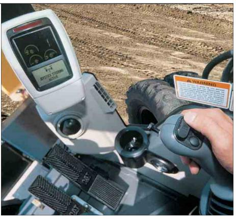
**Power Modes.** There are three power mode settings. The operator can choose the best power setting for both engine and hydraulic power versus fuel efficiency.
