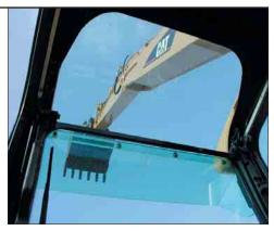
**Skylight.** A unique large polycarbonate skylight provides excellent upward visibility.
