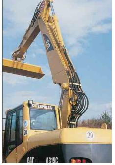
**Hydraulic Cylinder Snubbers**. The hydraulic cylinder snubbers at the rod end of boom cylinders, both ends of stick cylinders and bucket cylinder rod end cushion shocks, reduce sound and increase cylinder life, keeping the machine working longer.
