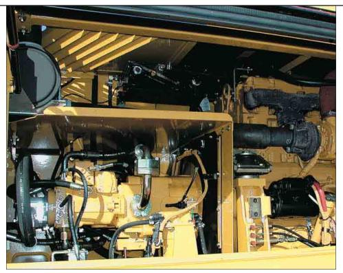
**Ground Level Service.** The design and layout of the M315C was made with the service technician in mind. The fuel water separator, engine oil filter, battery, radiator fluid level, fuel filter, engine oil gauge, hydraulic oil level, air cleaner and pilot system filter are all easily accessible at ground level allowing critical maintenance to be done quickly and efficiently.
