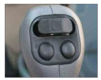
Adjustable Hydraulic Sensitivity. It allows the operator to adjust the aggressiveness of the machine according to needs. For precision work, one of four different levels of aggressiveness can be pre-selected on the soft-switch panel. Increased sensitivity can then be quickly activated and deactivated during the work cycle by using the joysticks.
