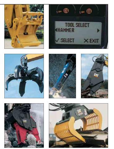
**Multi-Processor.** The Caterpillar Multi-Processors can be equipped with different jaw types depending on your need.
