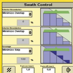
**Sectional Control** cuts input costs by reducing skips or overlaps dramatically. This GPS-based system turns boom sections on and off automatically whenever you leave or enter a predefined area.
