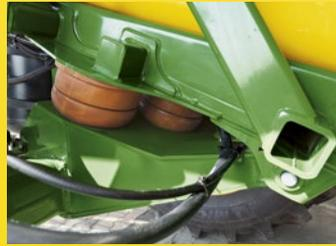
**ProRoad:** this double-link axle suspension system has special polyurethane dampers to absorb shocks on the road and in the field. For more comfort, greater spray accuracy and a longer sprayer life.
