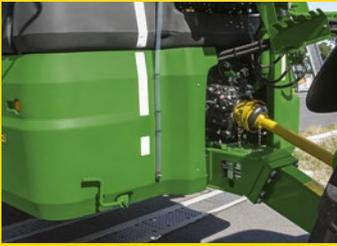
**Low-slung design:** The low centre of gravity and even weight distribution ensure safe, easy handling at speeds up to 40 km/h\*.
