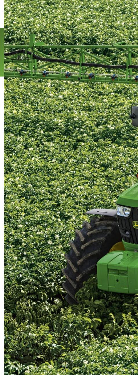
**John Deere section control** takes full control of the boom sections, automatically switching them on and off when you leave or enter predefined areas and also the headland.
