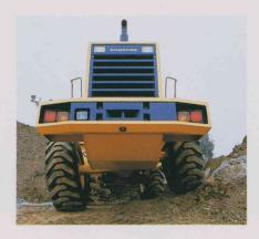
High machine stability is assured by a center-pin-supported rear axle and large oscillation angle that keep the machine level on even the roughest surfaces. This, plus a long wheelbase, wide tread and large static tipping load, give Komatsu wheel loaders high stability for efficient digging/carrying operations. In addition, torque proportioning differentials (installed on models WA100 through WA470) minimize tire slippage and extend tire life.
