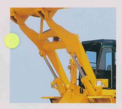
Z-bar loader linkage ensure greater breakout force and provide a longer dumping reach and clearance, boosting productivity and facilitating access to dump trucks. They also contribute to excellent front views, making it easy to conduct leveling work.
