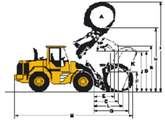
L60F L60F Sales code: WLA82194 Operating weight (incl. logging cw 120 kg): 12 210 kg Operating load: 3450 kg
