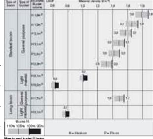
The size of rock buckets is optimized for optimal penetration and filling capability rather than the density of the material.
