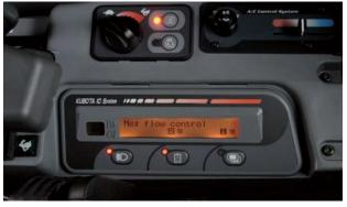
The unique Kubota Intelligent Control System gives you precise control of oil flow according to your needs or the attachment in use.
