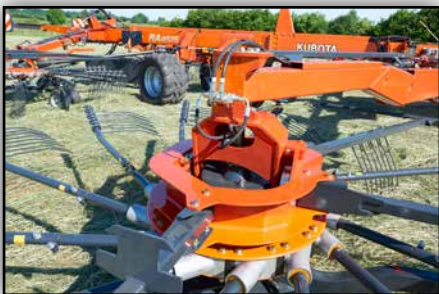
Each rotor can be independently and hydraulically set for height. As well a minimum height can be mechanically adjusted to secure a correct setting.
