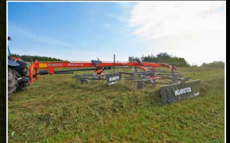
The low position of the rear frame ensures excellent stability.
