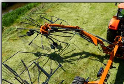
The two outer rotors can be adjusted individually to match a working width between 9.50-15.00m.
