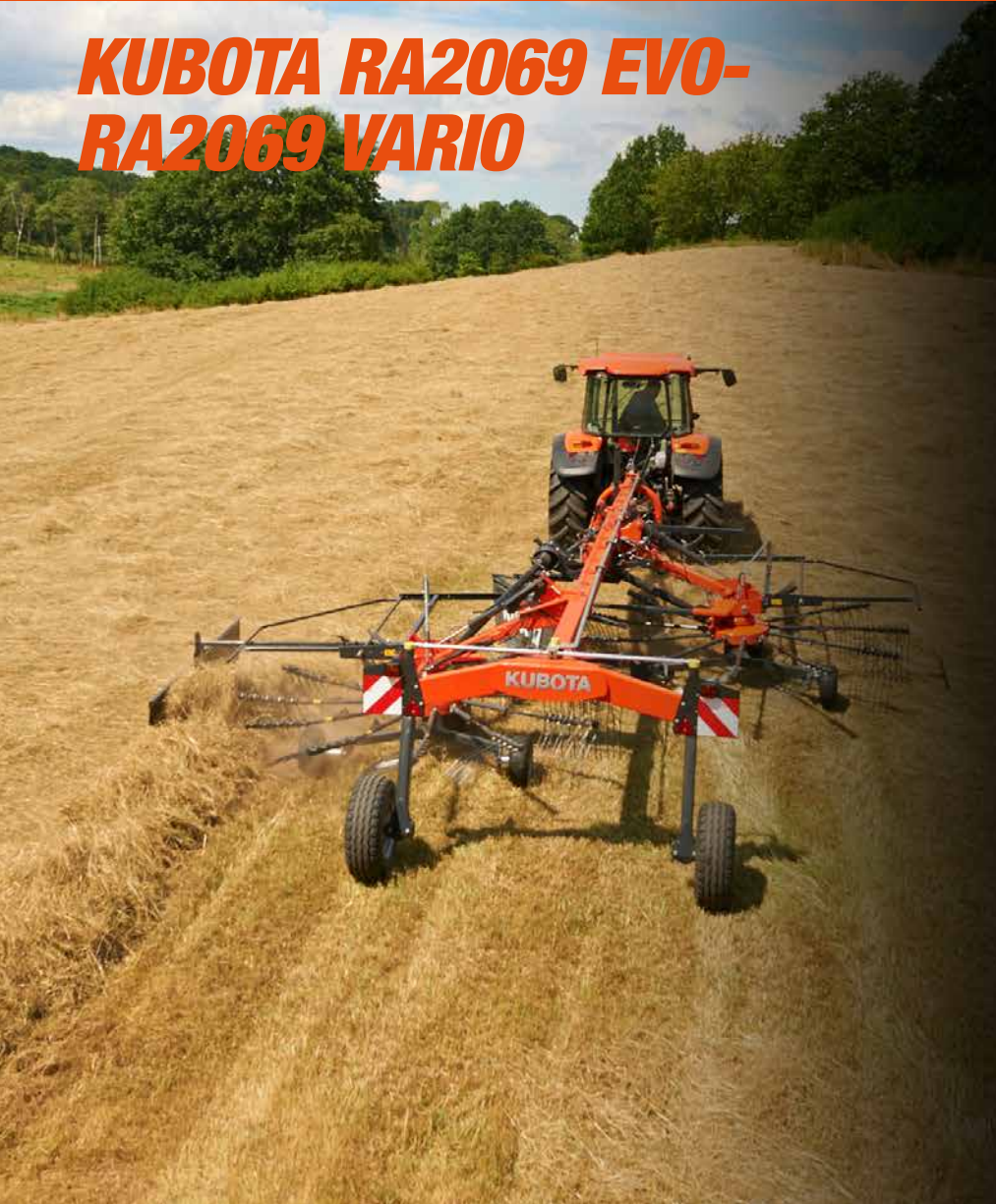
Generous overlap between rotors ensures clean raking.
