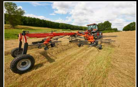
The VARIO version offers the possibility of raking two separate swaths.
