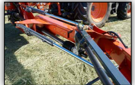
Hydraulic suspension of front lift arm and BreakBack system.
