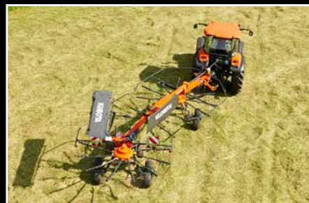
SideShift to the left - raking without driving on unraked crop.
