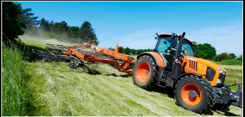
The unique elbow construction positions the front rotors close to the driver for excellent overview.
