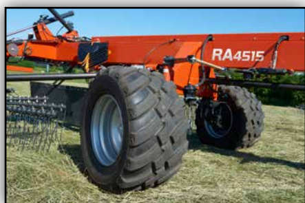
The optional active steering wheel provides excellent manoeuvrability during narrow gateways and tight corners.
