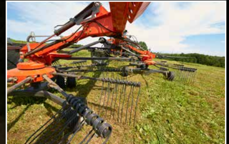
Generous overlap between rotors ensures clean raking.
