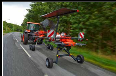
Pulled axles for smooth running characteristics and reduced power requirement.
