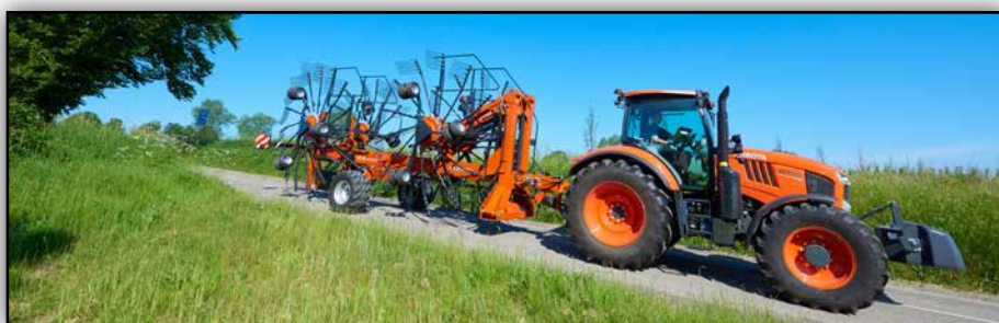
With its' clever folding mechanism the total height remains below 4.00m - despite a rotor diameter of 3.85m. And there is no need to remove tine arms for road transport.
