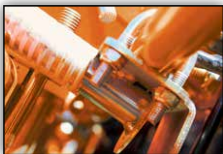
The position of the distribution outlet is before the roller. Position and angle are adjustable.
