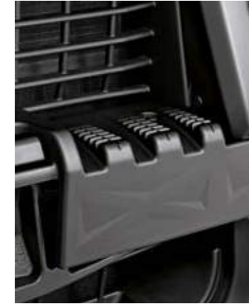
WINDSCREEN ACCESS STEPS non-slip to make servicing the vehicle easier.
