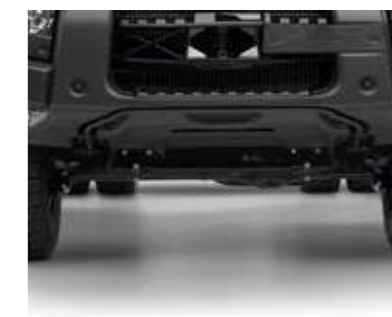
GUARD PLATE underneath the radiator and oil sump.
