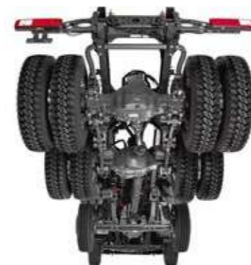
DOUBLE REDUCTION TANDEM DRIVE AXLE for greater traction on difficult terrain.
