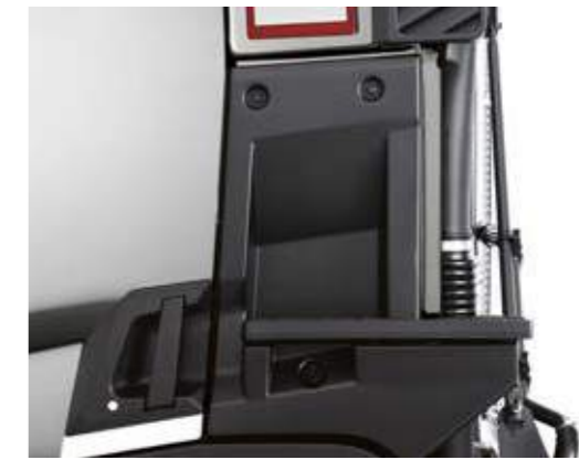
BODYWORK SIDE ACCESS STEP for ease of checking load content.
