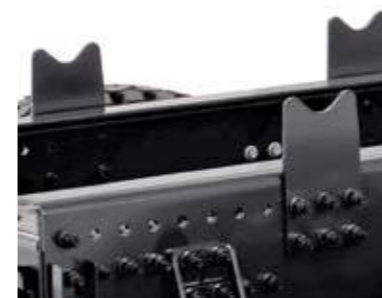
MOUNTING BRACKETS/PLATES ON SIDE MEMBERS for easier body mounting.
