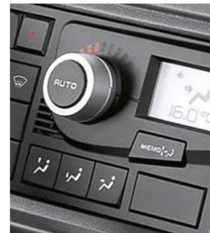
AIR CONDITIONING AND AUTOMATIC DE-ICING of the side windows, windscreen and rearview mirrors.
