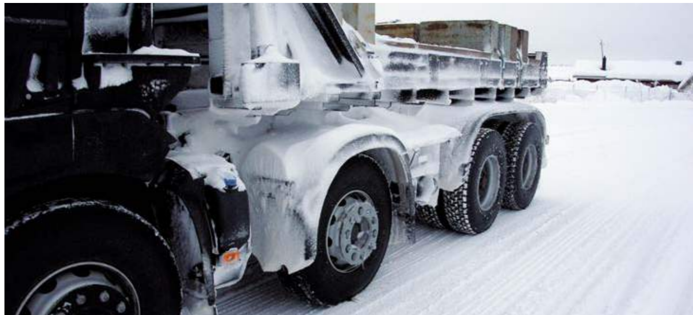
COLD-WEATHER TEST over several thousand km north of the Arctic Circle (Sweden).
