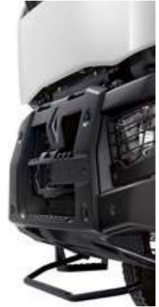
WINDSCREEN ACCESS STEPS non-slip to make servicing the vehicle easier.
