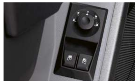
MANAGEMENT OF SIDE REARVIEW MIRRORS AND WINDOWS one-touch window lift and electrical adjustments for main and wide-angle rearview mirrors.
