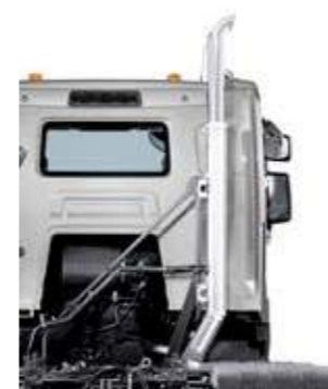
VERTICAL OUTLET for better body mounting options.
