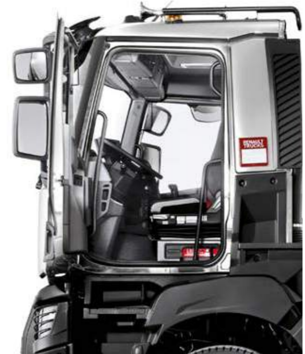
DOOR OPENING ANGLE 85° for easier cab access.
