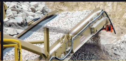
High production conveyor with belt cleaner
