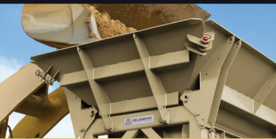
Hopper Capacity 8.0 m 3 (10.5 yd 3 )
