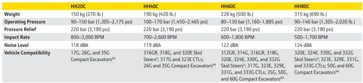
Mounting Bracket 9800 (17G), 9801 (26G and 35G), or 9802 (50G and 60G) required. All older mounting brackets will not interchange.
