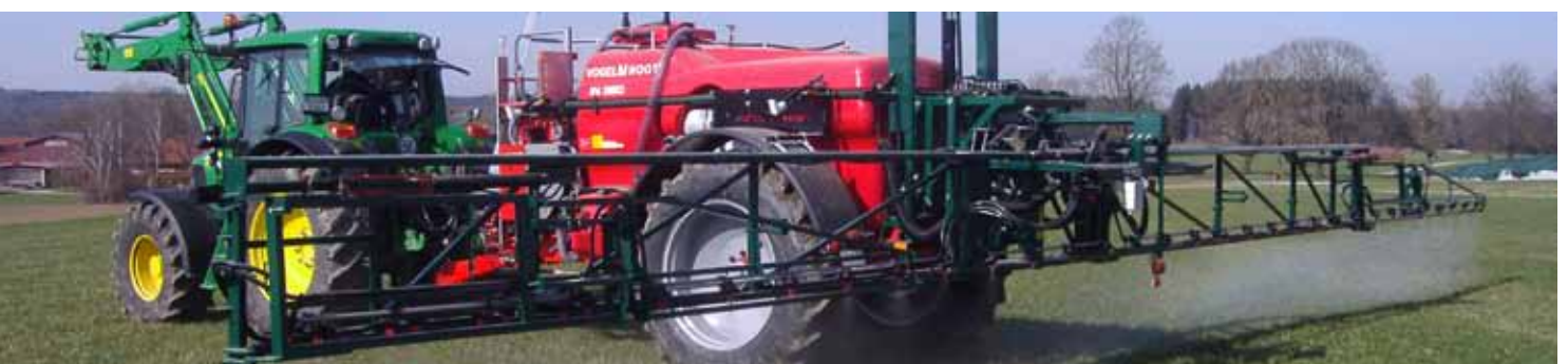
FH 903 piping (linkage) with asymmetric folding system
