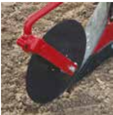
Disc coulters are available plain, notched or rippled, spring loaded or fixed.
