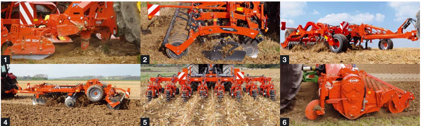
1. Soil looseners - 2. Compact disc harrows - 3. Stubble cultivators - 4. Disc harrows - 5. Strip-till tools - 6. Power tillers
