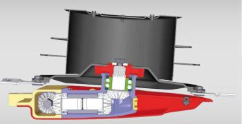
Cross-section of the cutter bar
