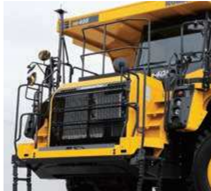
Safe cab access thanks to the low angle of the front stairways with handrails, slip-resistant
