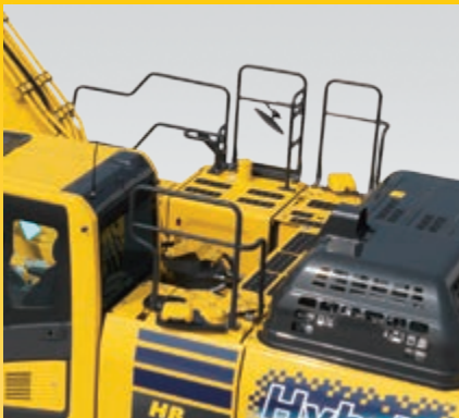
Hand rails and anti-slip plates
