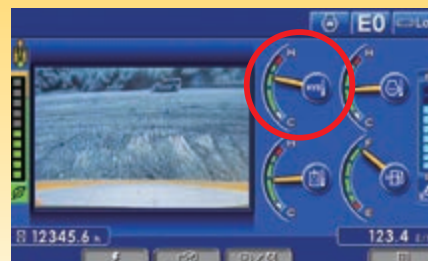
Hybrid system temperature gauge
