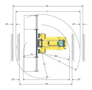
Ast = Practical 90 degrees Stacking aisle = V (theoretical stacking aisle) + a (total
