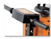
Adjustable anti vibration handles for operators comfort
