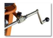
Cutting depth adjustment by handwheel
