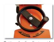
Cutting depth adjustment by handwheel
