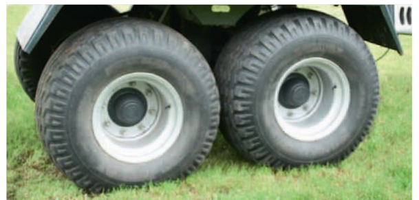
Bereifungsalternativen (Ackerstollenprofil 15/55-17, 380/55-17, 19/45-17, 500/50-17, 560/45 R 22.5).
