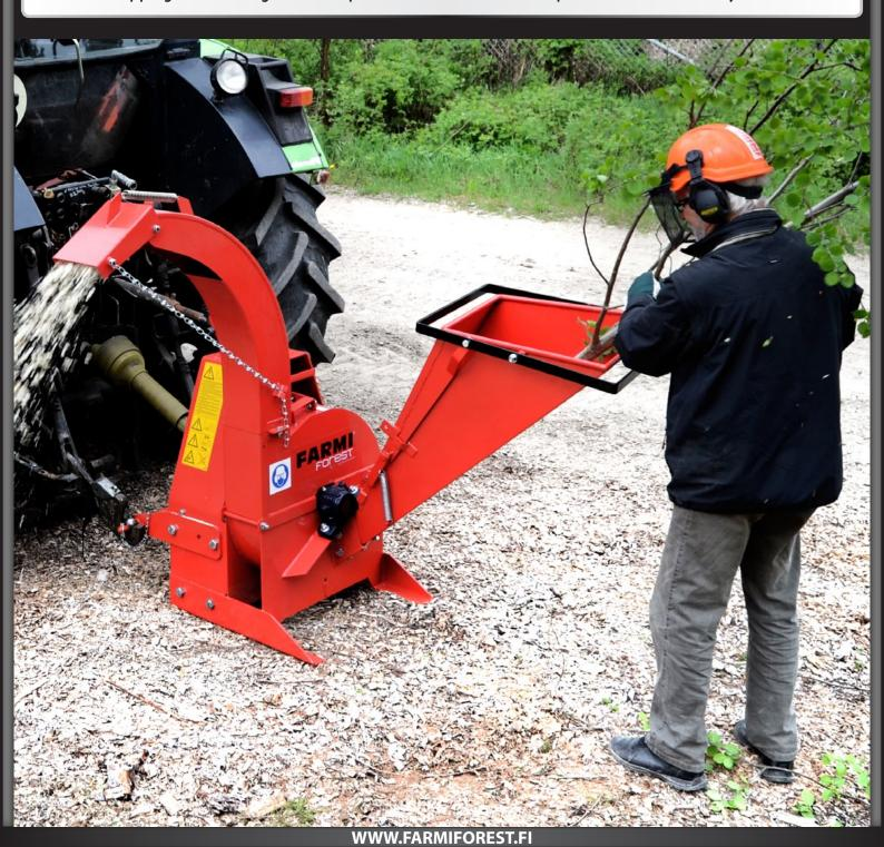
**FARMI CH 100 F** is designed as a robust and inexpensive disc chipper for landscaping to chip branches and small trees up to a diameter of 100 mm. The FARMI CH 100 F can be mounted onto a small tractor giving a compact chipping machine in gardens, parks, yards and road sides. Two knives and an anvil take care of chipping and feeding. CH 100 F chipper is available as a tractor PTO versions or as a hydraulic driven option.
