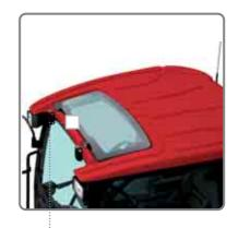
**Roof window** for excellent view of loader work and low clearances.
