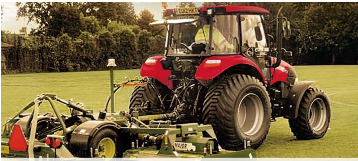
Non aggressive tread pattern tyres are suitable for sports pitch use.
